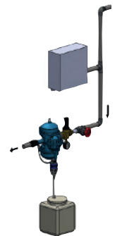
Tank Feed installation
