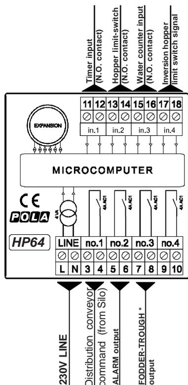
\* This contact closes at the start of the distribution and it is open when the distribution is completed (it can open with a delay time, see **Cost** function **t.man**).
